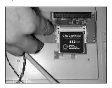
Mounting the Compact Flash IDE Adapter Inside the Intended Firewall
